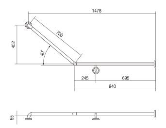
Drawn RH (Right Hand) Note: Horizontal flange connects directly to rear wall
